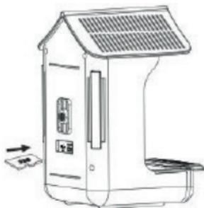
Note: Only when the TF card is inserted into the machine the machine can function normally. If the TF card is not inserted, the corresponding functions of the machine can not be used.
